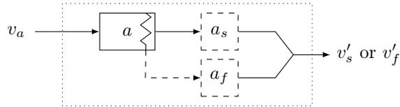
Figure 12: Dataflow diagram for the `try` combinator.
