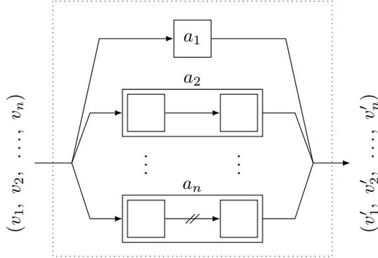
Figure 11: Dataflow diagram for the  $\mathbf{all}$  combinator over arrows  $a_1$  through  $a_n$ . The argument arrows can be simple or a complex result of other combinators ( $a_1$  and  $a_2$ , respectively), and can be synchronous or asynchronous ( $a_2$  and  $a_n$ , respectively).
